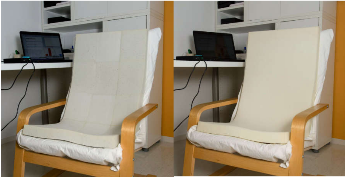
Figure 1: Biocrystal (left) and control (right) foam placed on a wooden chair during preparations for testing.
