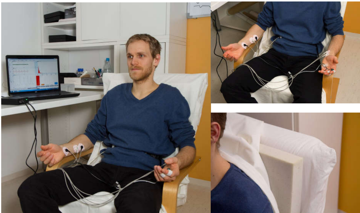
Figure 2: Demonstration of the testing set up. Testees were seated in a comfortable wooden chair (left) over which foam covered with cotton cloth was placed (lower right). Electrodes needed for measuring of physiological parameters were placed on both arms (upper right).
